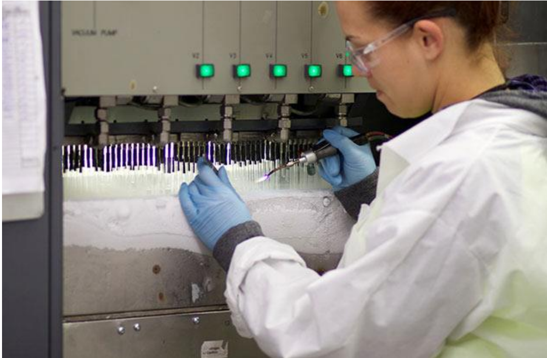
FIGURE 7: FILLING AND END-SEALING TRITIUM LIGHT SOURCES
